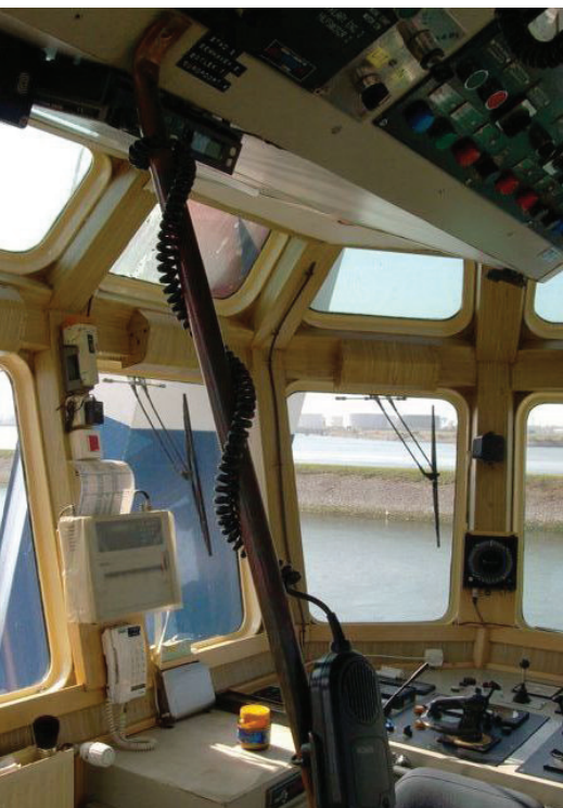
◀ Figure 4: Limited outside view from manoeuvring station.
