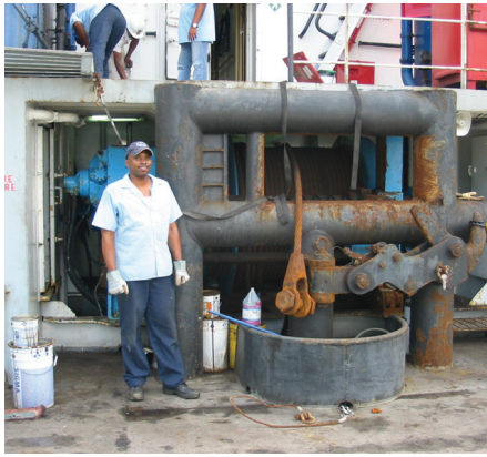
▲ Figure 6: A very high towing point, about 2m high.
