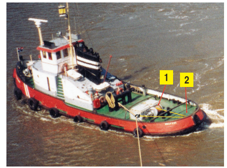
▲ Figure 5: Stern tug with gob rope (see yellow line aft). 1 = gob rope winch; 2 = swivel fairlead.
