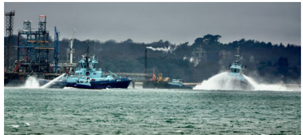
Tugs may use water monitors to disperse minor oil spills to help break down the pool.
