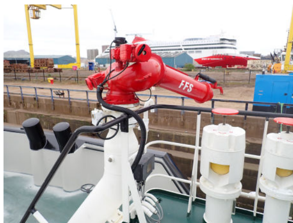
Tug with monitors at wheelhouse level
