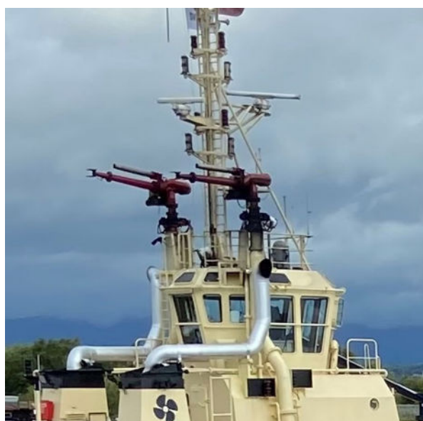
Tug with monitors positioned above the wheelhouse
