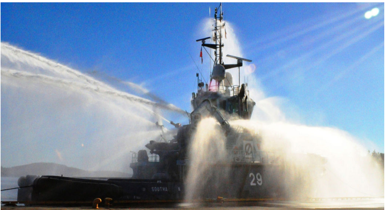
Tug showing full monitors and drenching systems activated - PHOTO CREDIT: NICK JEFFERY
